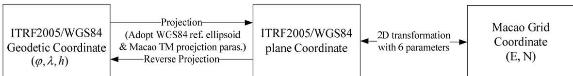
Coordinate transformation in 2D+1D is more rational than that in 3D, by which the converted coordinates are not affected by a deviation in the geodetic height, but it would be inconvenient to deal with plane coordinates and heights individually. Therefore, we also offer 3D transformation parameters between ITRF2005 and Macao Grid (Appendix 2) in order to cater for different users.
